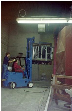
Forklift being narrowly prevented from tipping over by having an extra worker hop on the back of the forklift as a counterweight to prevent having the forklift and the load tip over.
